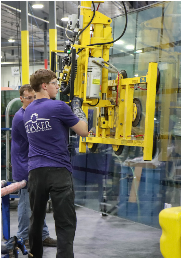
QUAKER USES glass manipulators (left) to move large glass units in the manufacturing facility. Chief Marketing Officer Bill Siffard said the equipment helps keep workers safe and prevent strain while working with heavy materials. "Number one for us is safety," he said.
